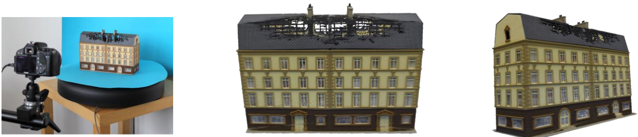
Figure 1: Turntable capture setup (left). Preliminary 3D reconstruction results of a miniature house model (middle/right)
