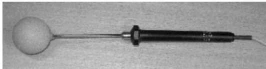
Fig 2. Globe thermometer consisting of a grey 38 mm acrylic ping pong ball around a Pt100 temperature probe [16]
