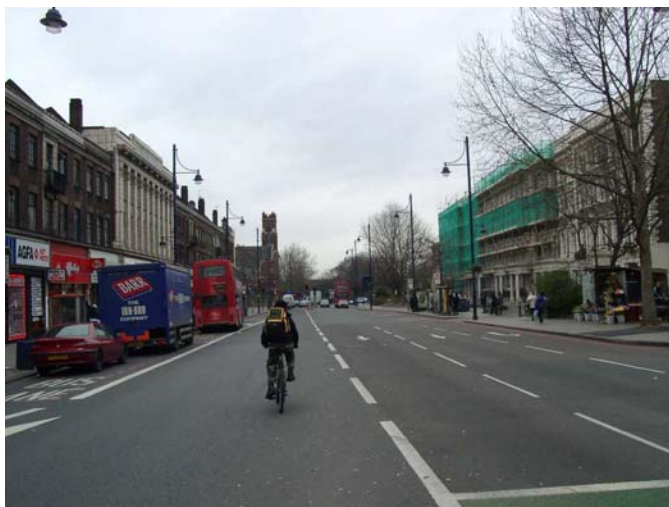
Wider running carriageway – suitable where there is a higher value of link status relative to place status
