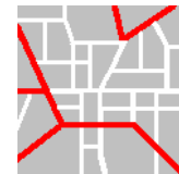
Strategic network too sparse. Although minimising route length, not so efficient as a connective network.
