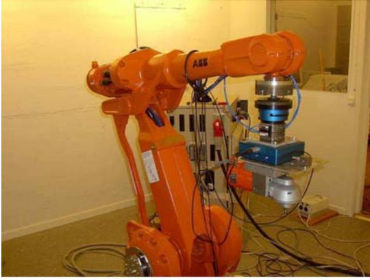
Fig. 2. The experimental setup. An ABB industrial robot IRB 2400 with an open control architecture system is used. The wrist sensor is placed between the robot tip and an compliance tool where the grinding tool is attached. The accelerometer is placed on the tip of the grinding tool.
