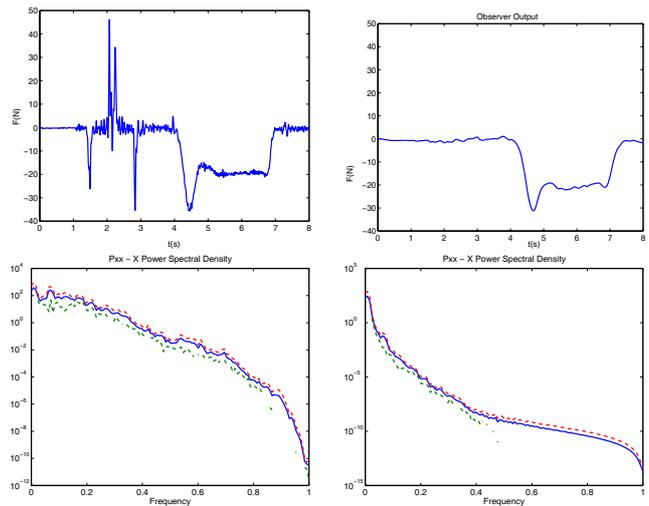
Fig. 5. Force measurement from the wrist sensor JR3 (upper-left), force observer output (upper-right), power spectrum density for the composed signal  $u - m\ddot{x}$  (lower-right) and observer output power spectrum density (lower-left). These results were obtained for z-axis.
