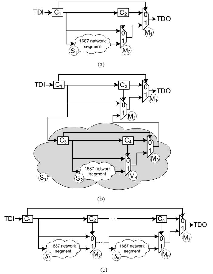
Fig. 3. Examples of MUX-based network used for computation of upper bound: (a) a network where the “1687 network segment” (i.e.,  $S_1$ ) can be an instrument shift-register or a network. (b) a network based on (a) where the “1687 network segment” is replaced with entire network in (a). (c) a generic structure in which “1687 network segment” parts can be replaced by the network in (a) to create a hierarchical MUX-based network.
