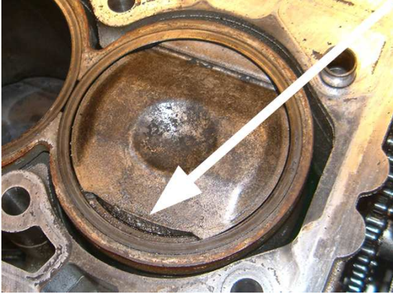
Figure 7: Damaged piston due to high PCP
