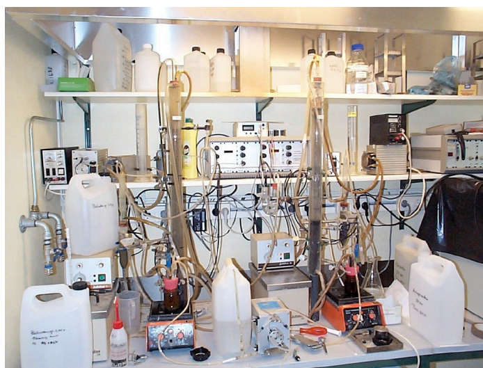
Figure 5.3 The two anaerobic fluidised reactors used in the experiment.
