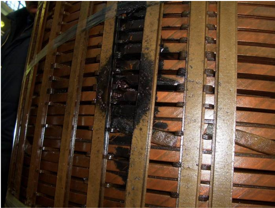
Figure 108: 35kV winding internal fault in phase L2.
