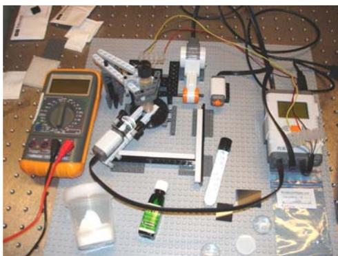
*Fig. 4.4.5. Automated polarimetric goniometer made from inexpensive LEDs, film polarizers, LEGO and controlled by a LabView compatible Mindstorm micro-processor. The setup was assembled during an exercise on scattering from powdered milk during a workshop in Lima, Peru<sup>346</sup>.*
