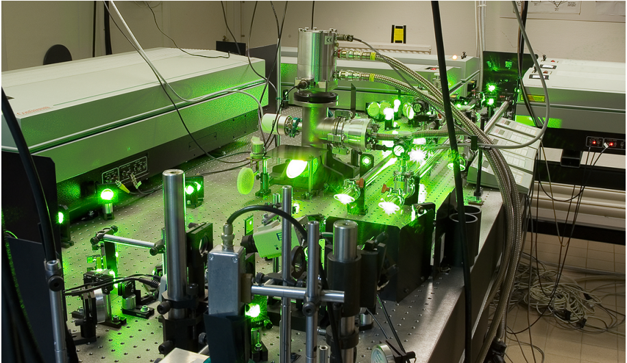
Figure 2.2: A photograph of the final amplifier of the multi-TW laser system when pumped by 5 frequency-doubled YAG lasers, each giving 1 J. The Ti:sapphire crystal is inside the housing of the cryogenic cooler.
