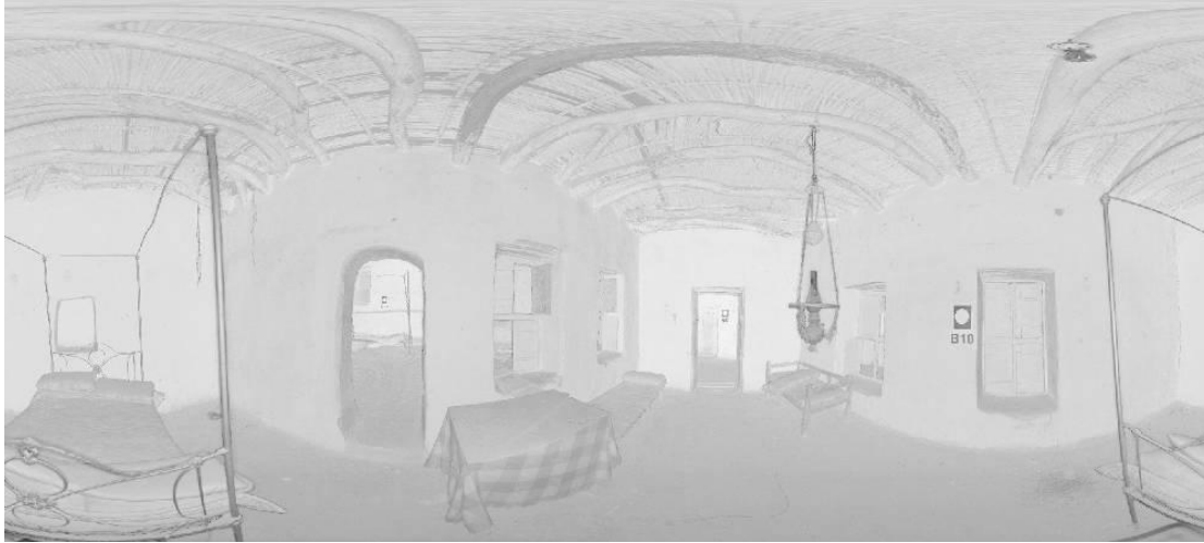
Figure 3: Laser scanning measurements were used as experimental measuring tool in Balat. One can get accurate measurements for vernacular buildings compared to manual sketches.
