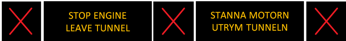
Figure 6. Benchmark design of the TIS used for the evaluation of the 11 TIS designs using the Theory of Affordance.
