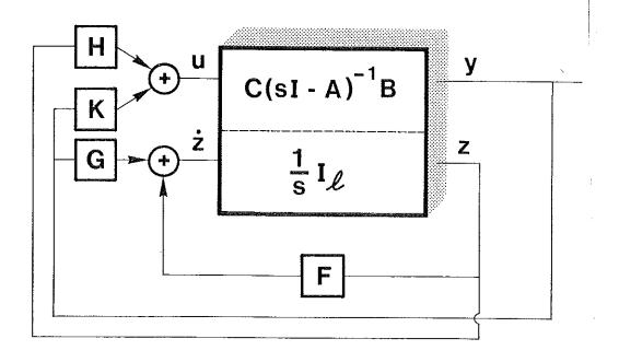
Figure 1. Dynamic feedback considered as static feedback.
