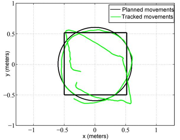
Fig. 4. Positioning results for circular and square movements.
