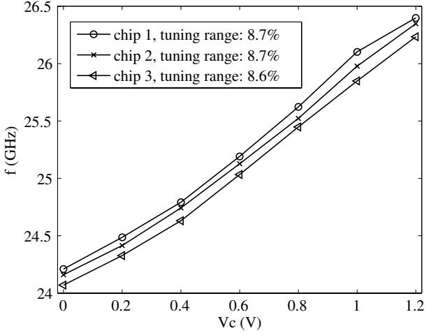
Fig. 3. Frequency vs. control voltage
