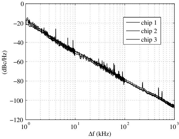
Fig. 5. Phase Noise vc. offset frequency,  $V_c=0.6$  V
