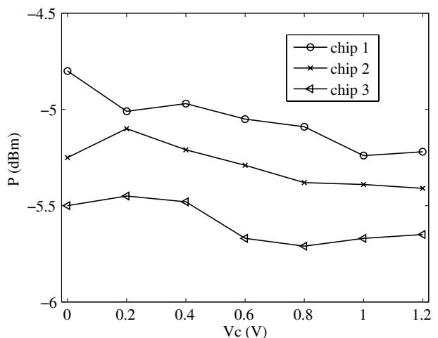
Fig. 4. Output power vs. control voltage
