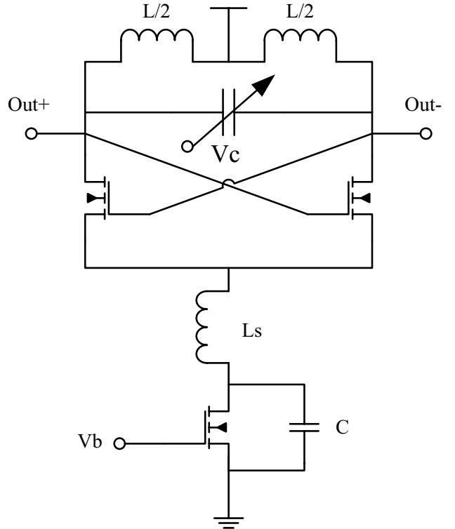
Fig. 1. VCO Schematic
