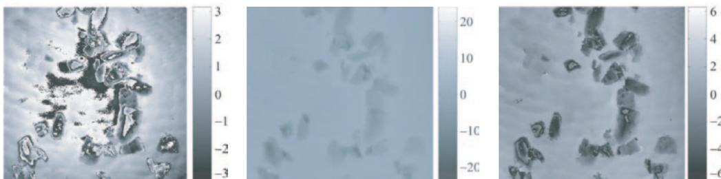
**Figure 4:** Phase images of lactose crystals mounted in a liquid with  $n_m = 1.570$ . The phase decreases when going from the liquid into the crystals. a) the wrapped phase image where the color changes from white over gray to black and back to white, modulus  $2\pi$ , in the crystals. b) the unwrapped phase image. c) the re-wrapped phase image.
