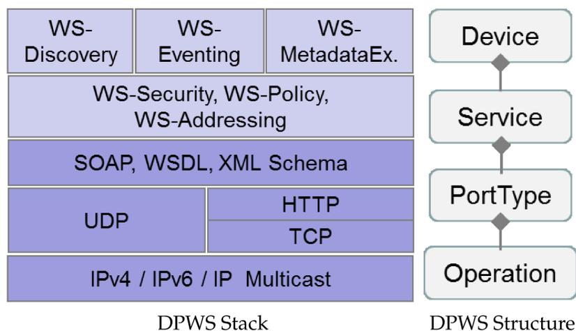
All DPWS devices are discoverable (WS-Discovery) and self-describing (WS-MetadataExchange), meaning that all information required to use a DPWS device can be obtained from the device itself, e.g. its IP-address, operations, and operation signatures.
