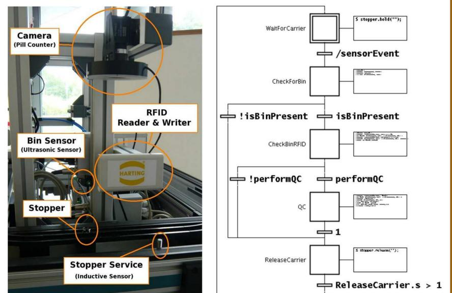
The DPWS implementation in Grafchart was tried out on a quality control station of SmartFactory<sup>KL</sup>'s SOA demonstrator, checking if bins have been filled with the correct number of pills.
