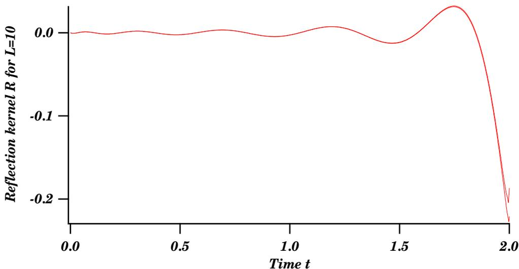
**Figure 3:** The reflection kernel  $R_{10}(1, s)$  for  $0 \leq s \leq 2$  using  $N = 2048$  and  $N = 4096$  spatial steps. Slight discretization error due to oscillations in  $a_L$  and  $b_L$  is evident.
