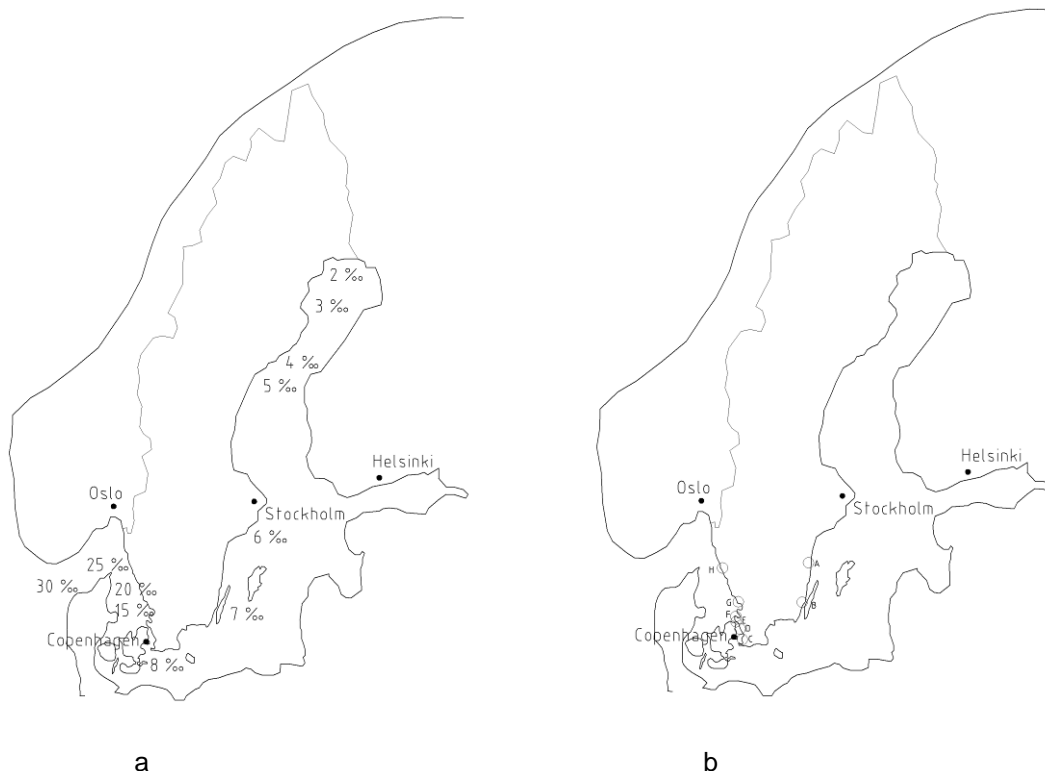
Figure 5: The salinity (‰) in sea water along the coast of Sweden (5 a) and locations of investigated harbors (5 b)
