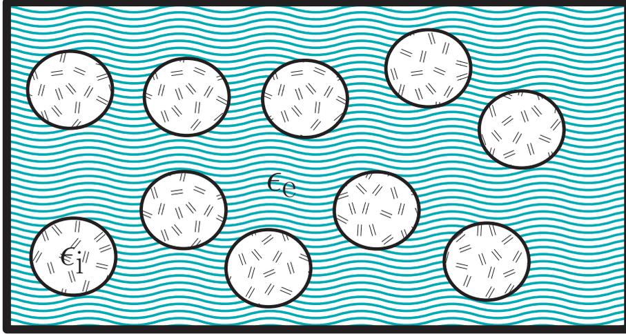
**Figure 1:** The homogenization problem: dielectrically anisotropic spheres embedded in anisotropic environment.
