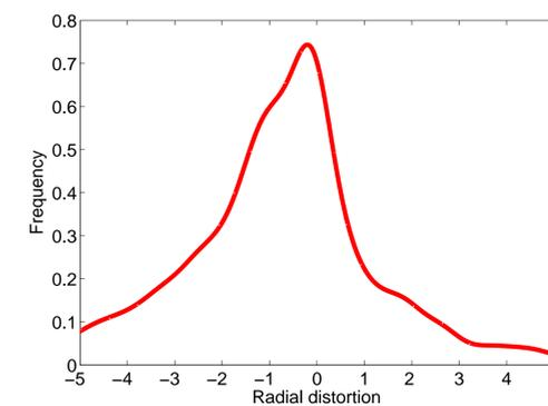
FIGURE 4: Result of kernel voting for radial distortion. The standard deviation of the Gaussian kernel was fixed to 1/3 and the peak of the curve is at  $\mu = -0.20$ . This value was used to remove distortion from the image. In Figure 5 the result after rectification is shown.
