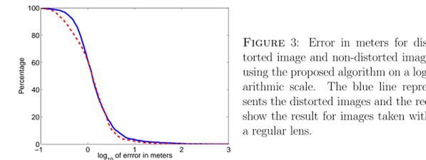
FIGURE 3: Error in meters for distorted image and non-distorted image using the proposed algorithm on a logarithmic scale. The blue line represents the distorted images and the red show the result for images taken with a regular lens.
