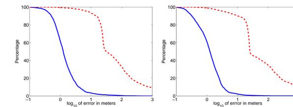
FIGURE 2: The percentage of images with an estimated position further away than a given distance to the position given by Photo tourism. The error is roughly given in meters. Notice the logarithmic scale. The blue solid line is for the proposed method and the red dashed represents the method without distortion. The left plot is for the fisheye lens and the right is for a regular lens.
