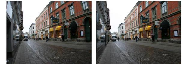
FIGURE 5: Left: An image taken with a fisheye lens. Right: The same image rectified after kernel voting was used to determine the radial distortion
