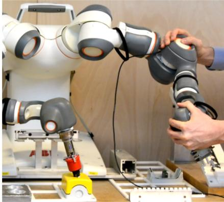
**Figure 8.1** Example use case of the proposed interface. An operator demonstrates a peg-in-hole task by moving the left robot arm through physical contact. The right robot arm follows the demonstrated movement in real time.
