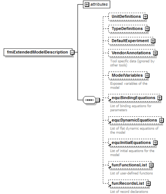
Figure 2. Overall structure of the DAE XML schema
