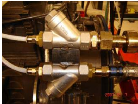
Figure 37 Pressurized air switching system built up by the check valves.
