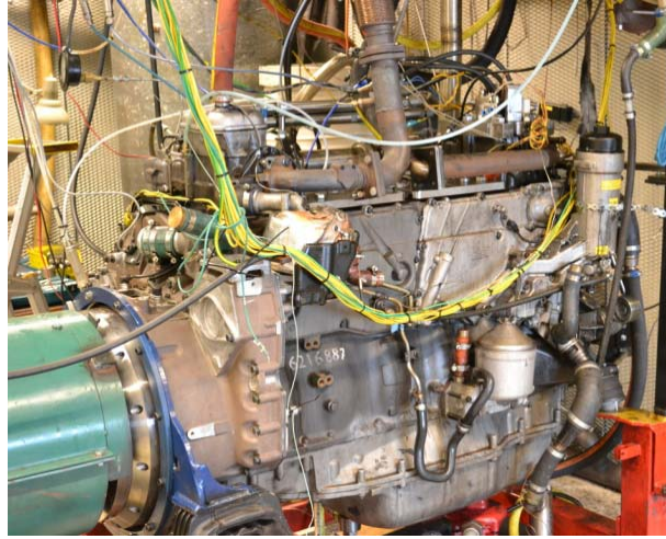
Figure 35 The modified Scania D13 Diesel engine. The operating cylinder is to the left in the picture
