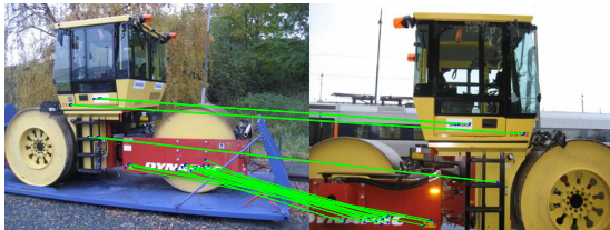
Figure 6.1: ROAD ROLLER. In this image pair, 28 seemingly correct correspondences (green lines) are obtained in the estimation of the epipolar geometry. Even though the epipolar geometry is plausible and perfectly valid, it does not correspond to the true geometry.
