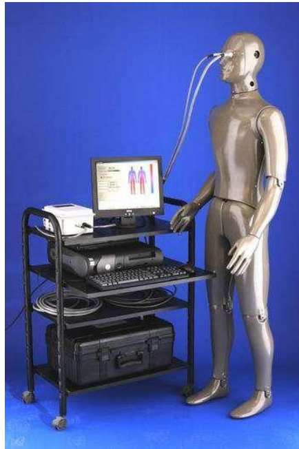
Fig.1 20-zone sweating thermal manikin “Newton”
