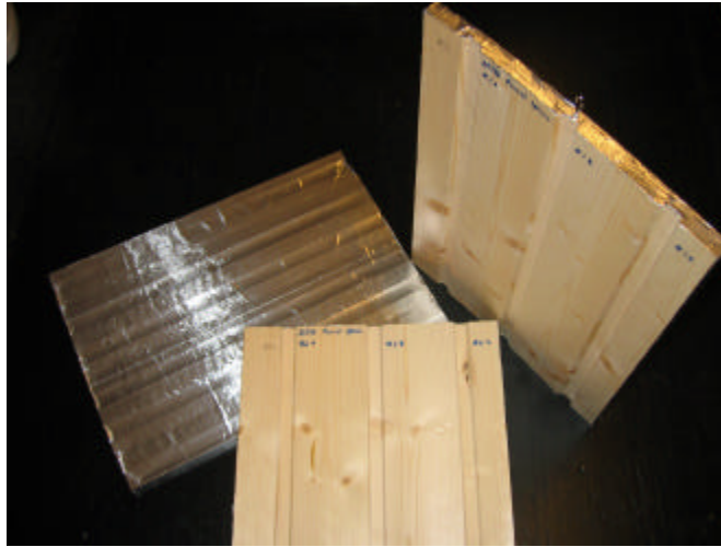
Figure 3 Picture of spruce panels after preparation so they are ready for test.
