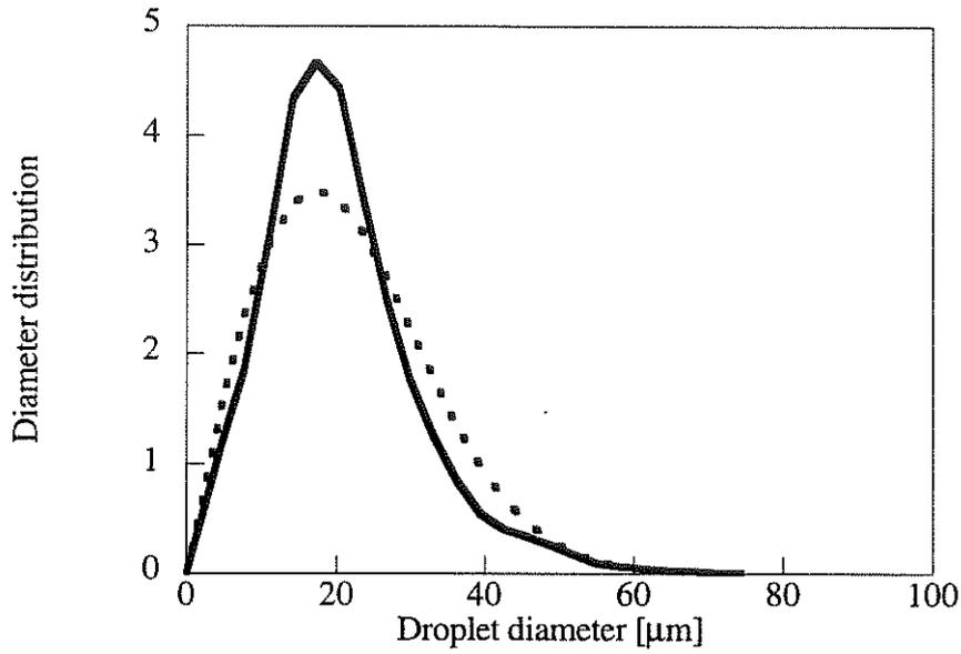
Figure 3 The droplet size distribution for the Lechler 212.085 nozzle at 80 bar and the predicted distribution using the Rosin-Rammler function (dotted line).
