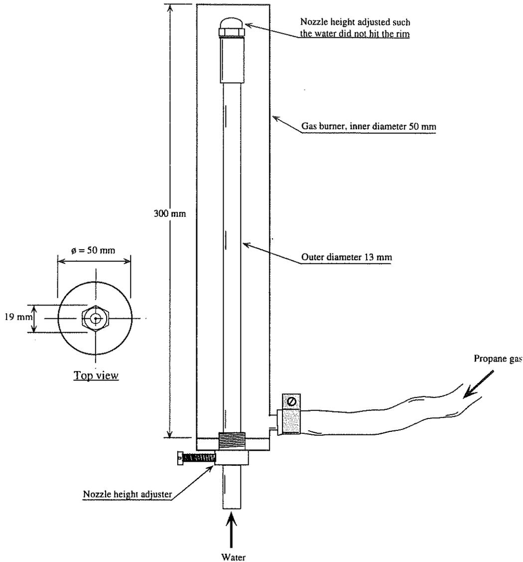
Figure 12 Detail of the tubular gas burner and the position of the water nozzle used in the REMP experiments
