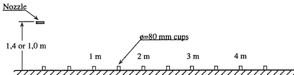
Figure 10 Principle sketch of the horizontal distribution measurements.
