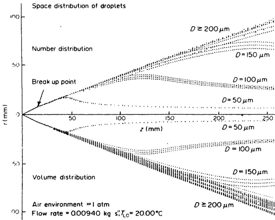
Figure 6 Example of a water spray pattern.
