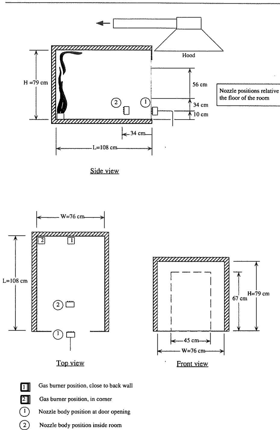
Figure 15 Principle sketch of the 1/3-scale room.
