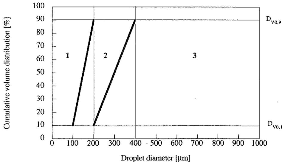
Figure 2 The definition and the division into different classes of water mist according to NFPA 750 [3].
