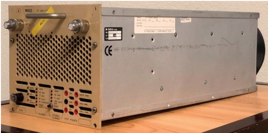
Fig. 3.13. The base-station amplifier with high linearity and high output power.
