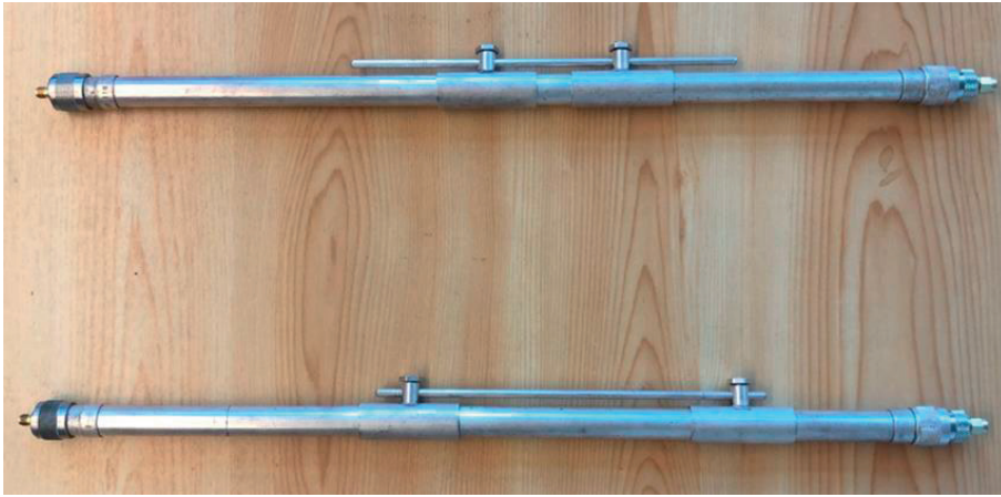
Fig. 3.11. The two additional impedance tuners, which are tuned manually.
