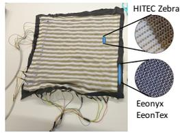
Figure 1: Pressure sensor matrix cover for ActivFOAM.
