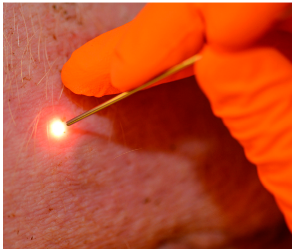
Figure 4. The thin DRS probe used to both deliver the incident light and collect the diffusely reflected light (see Paper II).
