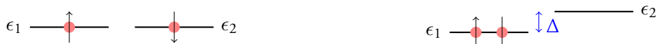
Figure 6.3: Detuning between the single electron energy levels in the quantum dots. The two-electron ground state changes when detuning the one electron levels. When the detuning becomes strong enough to overcome the Coulomb repulsion, the S(2,0) becomes the ground state.
