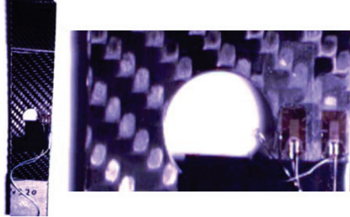
Figure 6 Test specimen (150 × 49 mm plate with hole of Ø20 mm) to establish material behaviour
