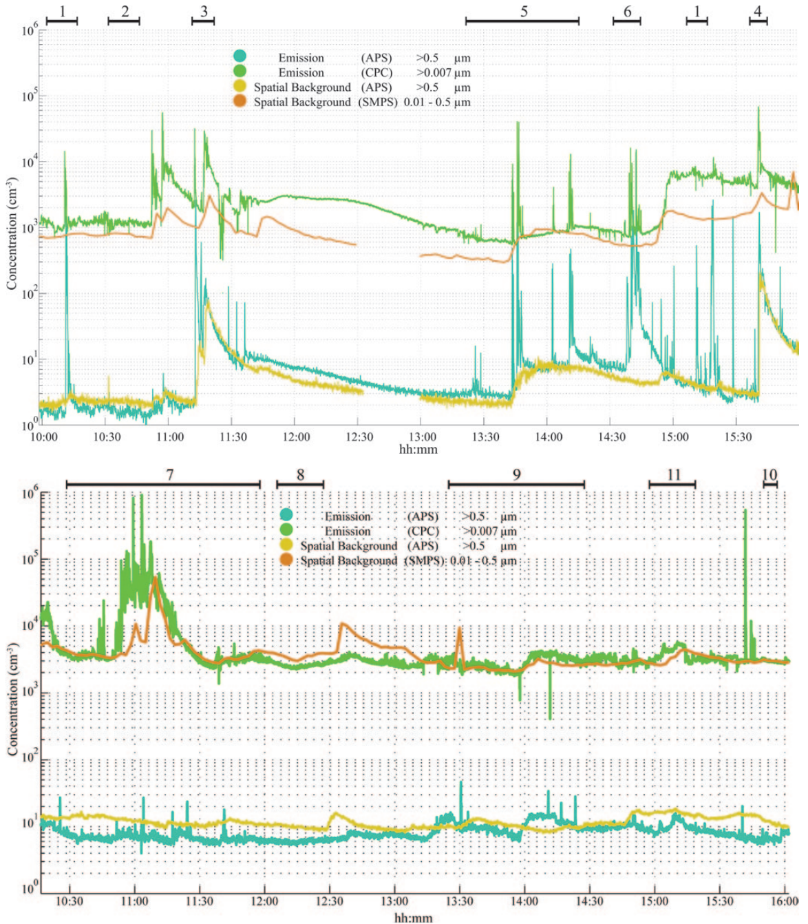
Figure 2 (a) Time series from online instruments measured in the production and sieving laboratories on the first day. Nos. 1–6 refer to Work Tasks: 1. Cleaning of deposits, 2. Harvesting, 3. Opening of the reactor, 4. Cleaning of the reactor, 5. Sieving, 6. Lathe machining. The numbers also refer to the locations in Table 1 and Fig. 1. (b) Time series from online (DRI) instruments measured in the purification laboratory on the second day. Nos. 7–11 refer to Work Tasks: 7. Purification Part I, 8. Purification Part II, 9. Functionalization Part I, 10. Functionalization Part II, 11. Grinding. The numbers also refer to the locations in Fig. 1.
