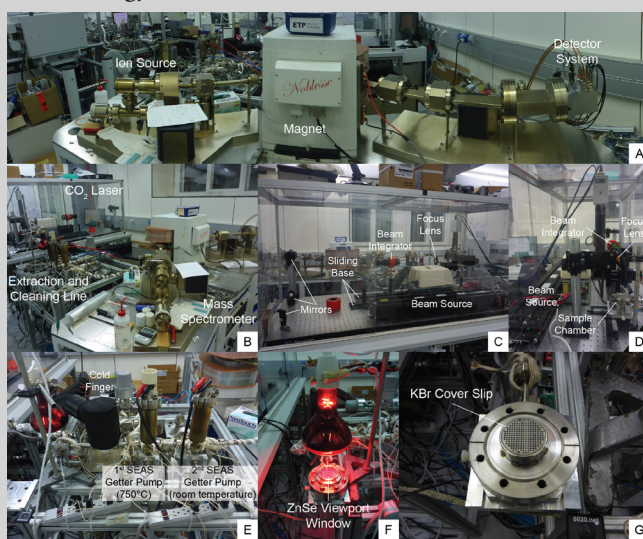
Figure Box 6.1 A) Nu Instruments Noblesse multi-collector noble gas mass spectrometer showing its three main components: left) ion source, centre) magnet, and right) detector system (photo: author of this thesis, 10/01/2018). B) Instrumentation set-up in the Quaternary Dating Laboratory (Quadlab), Natural History Museum of Denmark in Copenhagen, showing the argon extraction line, equipped with a defocused 50-W Synrad \text{CO}_2 laser to the left, as well as the fully automated Nu Instruments Noblesse multi-collector noble gas mass spectrometer to the right (photo: author of this thesis, 10/01/2018). C) 50-W Synrad \text{CO}_2 laser from the side (photo: author of this thesis, 10/01/2018). D) 50-W Synrad \text{CO}_2 laser from the front showing where the sample chamber for the argon extraction is situated (photo: author of this thesis, 10/01/2018). E) Gas cleaning system consisting of a cold finger to freeze the \text{H}_2\text{O} and two SAES GP-50 getter pumps to remove the hydrocarbons and \text{H}_2 , respectively (photo: author of this thesis, 10/01/2018). F) Sample chamber with the ZnSe viewport window which transmits the infra-red radiation of the laser beam. The sample chamber is baked under continuous pumping to re-establish the vacuum after the sample loading, where this part of the extraction line is exposed to atmospheric pressure (photo: author of this thesis, 10/01/2018). G) Opened sample chamber during sample loading. This part is exposed to atmospheric pressure. It shows the KBr cover slip right on the copper laser disc. The cover slip prevents that melted or evaporated sample material is introduced into the vacuum or condensate at the ZnSe viewport during the step heating (photo: author of this thesis, 10/01/2018).
