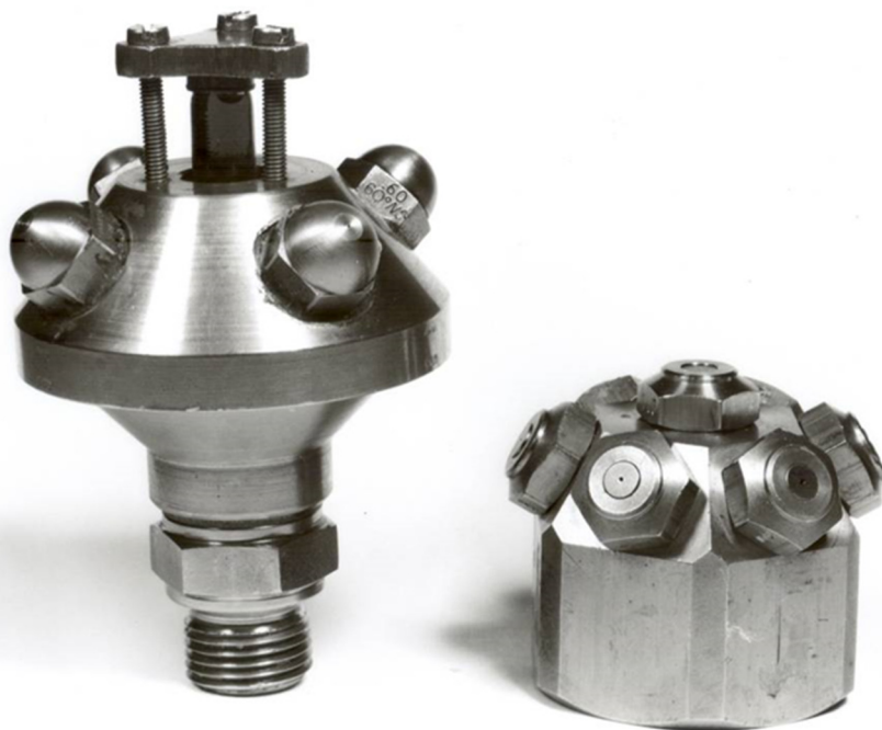
Figure 4 A very early automatic (with glass bulb) multi-orifice nozzle developed by HTC i Åmål AB along with a "1 7N2 Fogjet" nozzle from Spraying Systems Co. (to the right) that was tested at SP in 1983. Photo: Håkan Ungerth.
