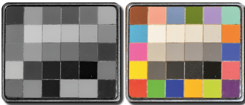
Figure 2.1: Monochromatic and multispectral images of an X-Rite Color Checker. The greyscale image has numerous squares with similar light intensity values which therefore appear the same and their colour cannot be discerned. The colour image combines red, green and blue light intensity making it possible to discern the different colours in the sample.
