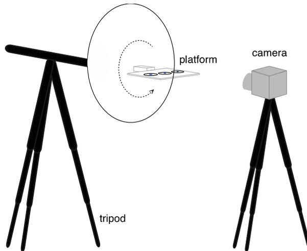
**Fig. 9** Experimental setup where bumblebees were trained to feed from three circles of filter paper, drenched in sugar solution, and placed on a flat platform that was attached to a rotatable arm on a tripod. The landings were filmed from the side by a high-speed camera. Adapted from Reber *et al.* (2016a)
