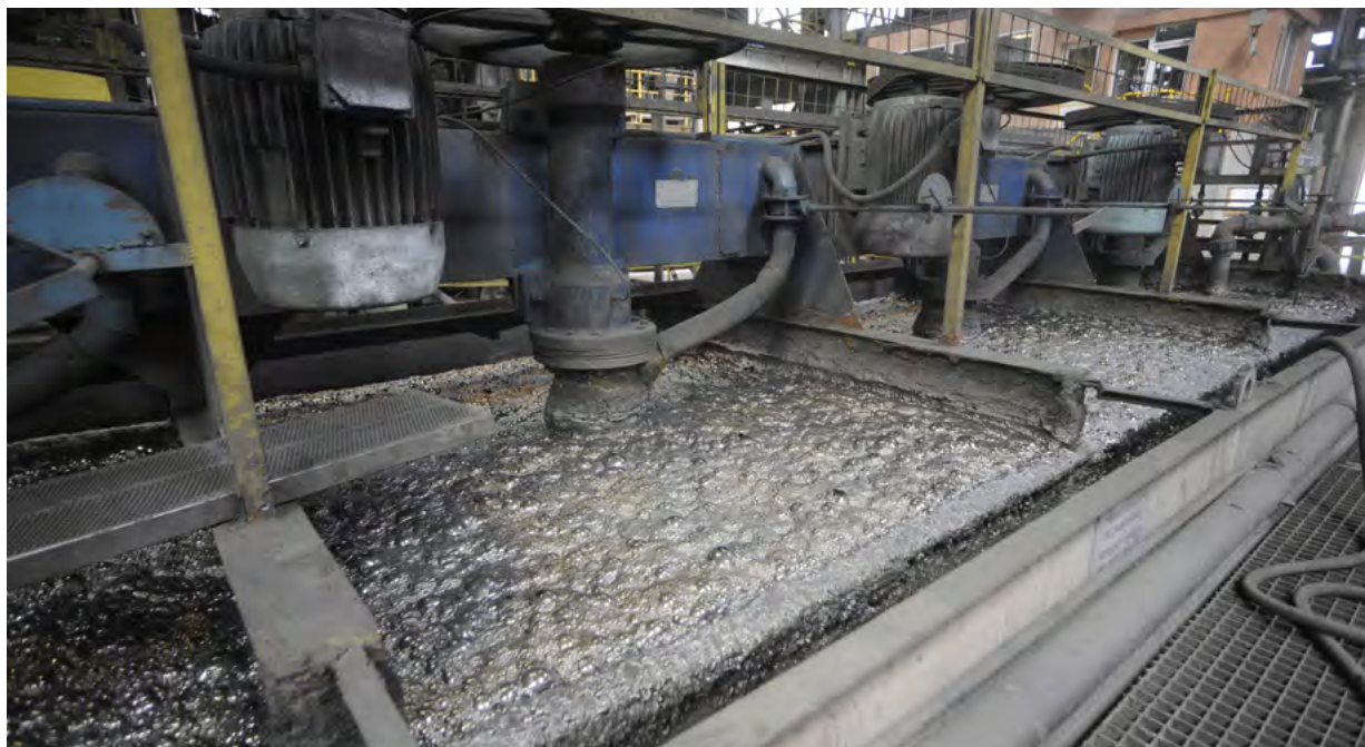
Figure 1.3 Flotation process to obtain metal concentrate.
