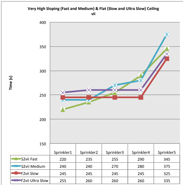
Figure 7-38: Sprinkler Activation Times for 33.69 ° Sloping Fast and Medium and Flat Slow and Ultra Slow Ceiling Models
