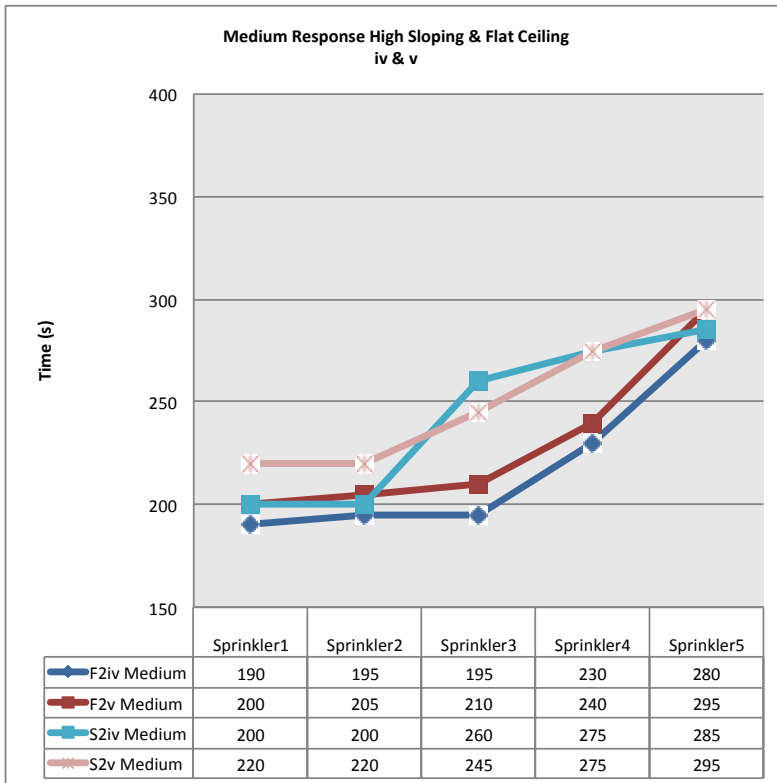
Figure 7-30: Sprinkler Activation Times for Medium Response High Sloping and Flat Ceiling Models
