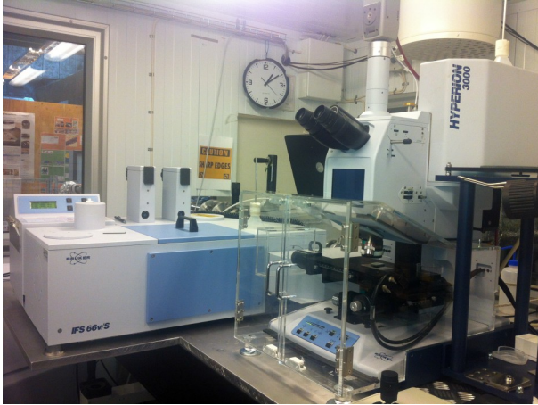
Fig. 6. Bruker IFS66/v FTIR spectrometer connected to a Hyperion 3000 microscope at MaxIV, Lund.
