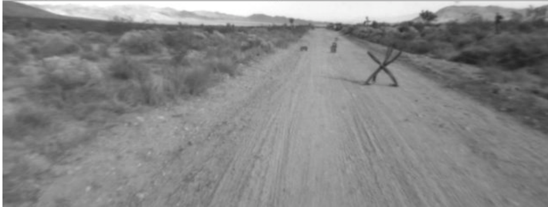
Figure 38: Obstacle detection and navigation test. The object to the right is a model of a so called Tank Trap . The smaller obstacles are crate lids.
