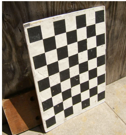
Figure 16: Old calibration target. Notice that the bottom left corner is slightly bent towards the camera.
