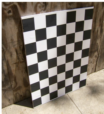
Figure 17: New calibration target. It is very flat, although it does not look so in this picture, due to lens distortion.
