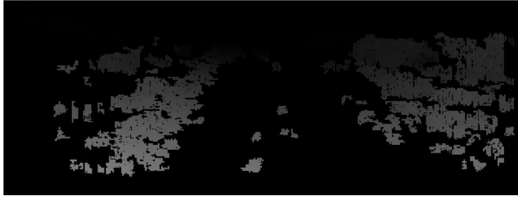
Figure 26: The disparity image from figure 24 after noise filtering. For this image, the filter's region size threshold is 50 and the connectedness tolerance level is 8.
