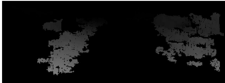
Figure 29: The disparity image from figure 24 after noise filtering. For this image, the filter's region size threshold is 350 and the connectedness tolerance level is 16.
