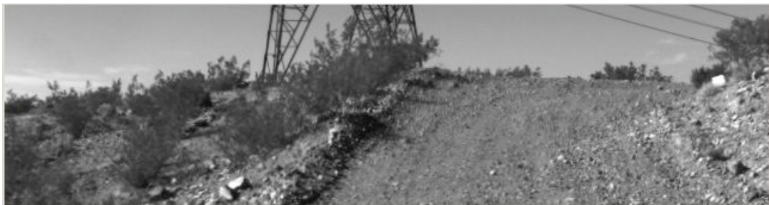
Figure 36: Left image from the long range cameras, dynamic subwindow is inactive. Alice's pitch is positive, resulting in the sky taking up a large portion of the image.
