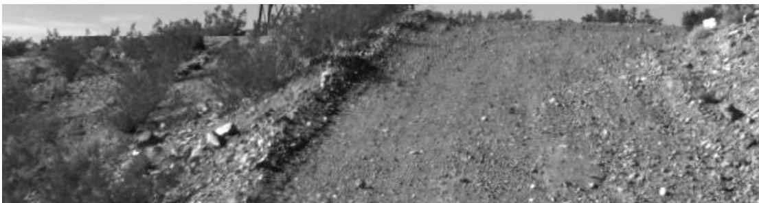
Figure 37: Left image from long range cameras, dynamic subwindow is active. The pitch is compensated for by vertical movement of the subwindow.
