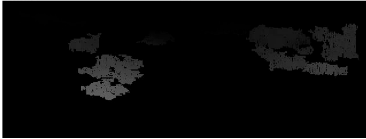
Figure 27: The disparity image from figure 24 after noise filtering. For this image, the filter's region size threshold is 1200 and the connectedness tolerance level is 8.
