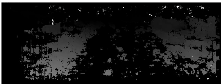
Figure 24: Disparity image from a desert road, with noise (brighter points are closer).
