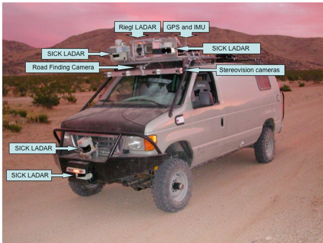
Figure 6: Alice, with terrain sensors marked.
