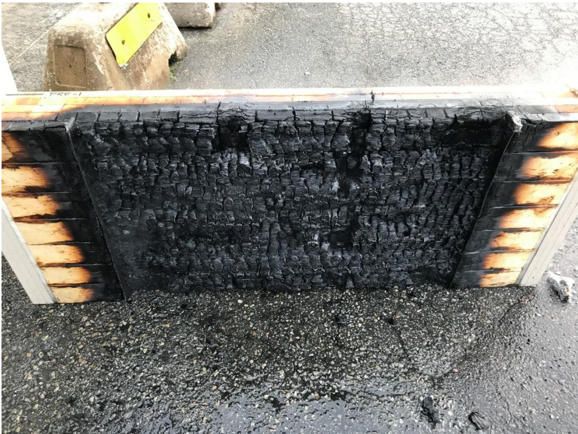
fig. G-13. The PRF-1 specimen, the day after the test. Very small pieces of char fell off the specimen during the test, but no delamination was observed. Overall the PRF-specimen performed well in the tests, with a steady and predictable fire development.
