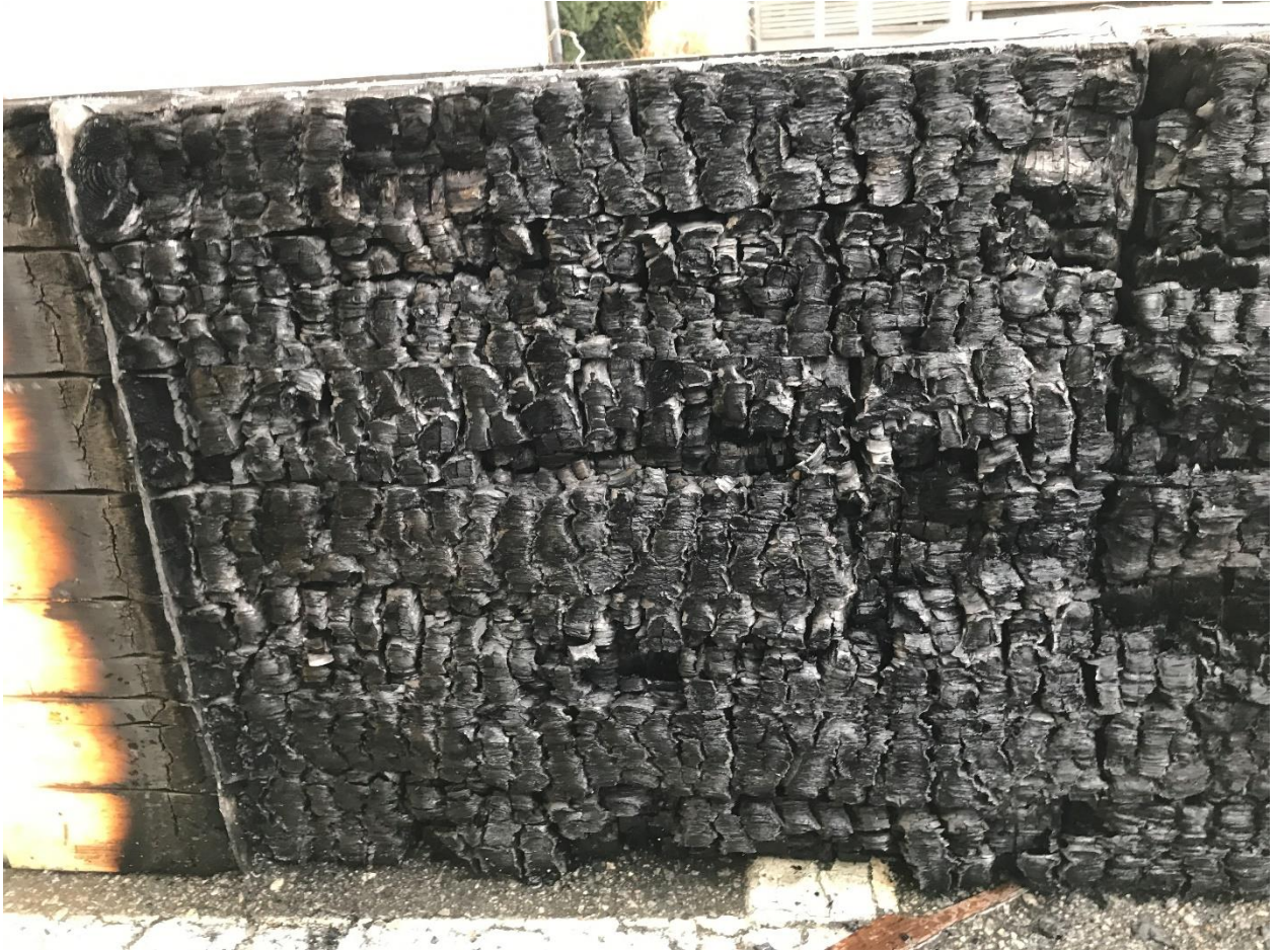
fig. G-14. Fire side of the MF-2 specimen the day after the test. The MF-specimen, just like the PRF-specimen, performed very well in the tests, and only minimal pieces of char fell off during tests.
