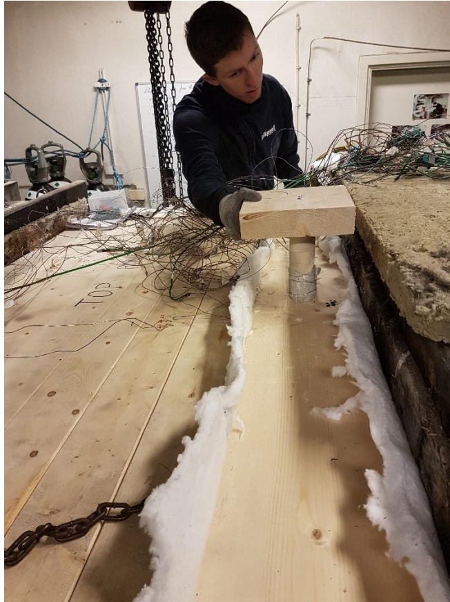
fig. G-27. Beam beside the specimen with a hole for the heat flux meter to be mounted in when in the furnace. In this picture Anton is placing a stopper to avoid fire and/or gases to spread up when heat flux meter is not used.
