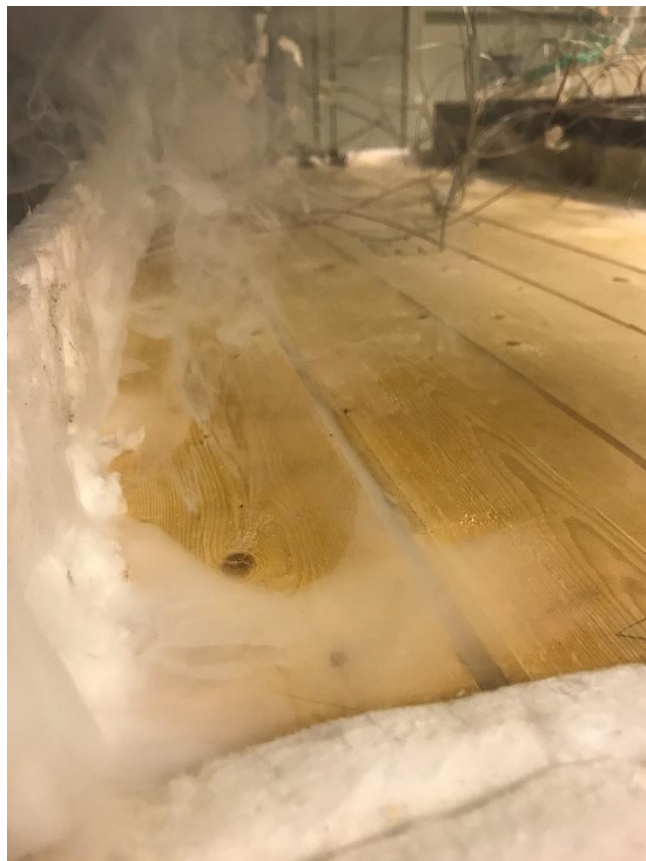
fig. G-6. Top side of EPI-2 specimen during experiment. In the initial heating phase of tests, moisture-rich smoke could be observed through the more severe gaps of the top layer of some specimen.
