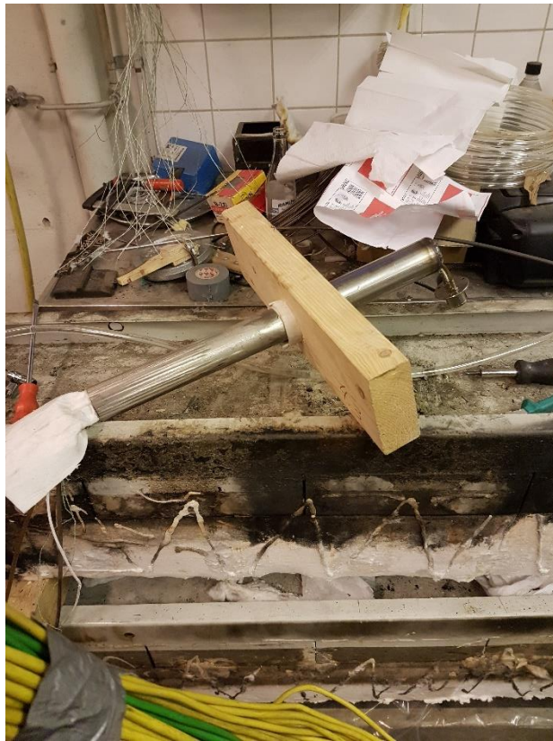
fig. G-26. Heat flux meter placed in a piece of wood for easy use during the experiments.
