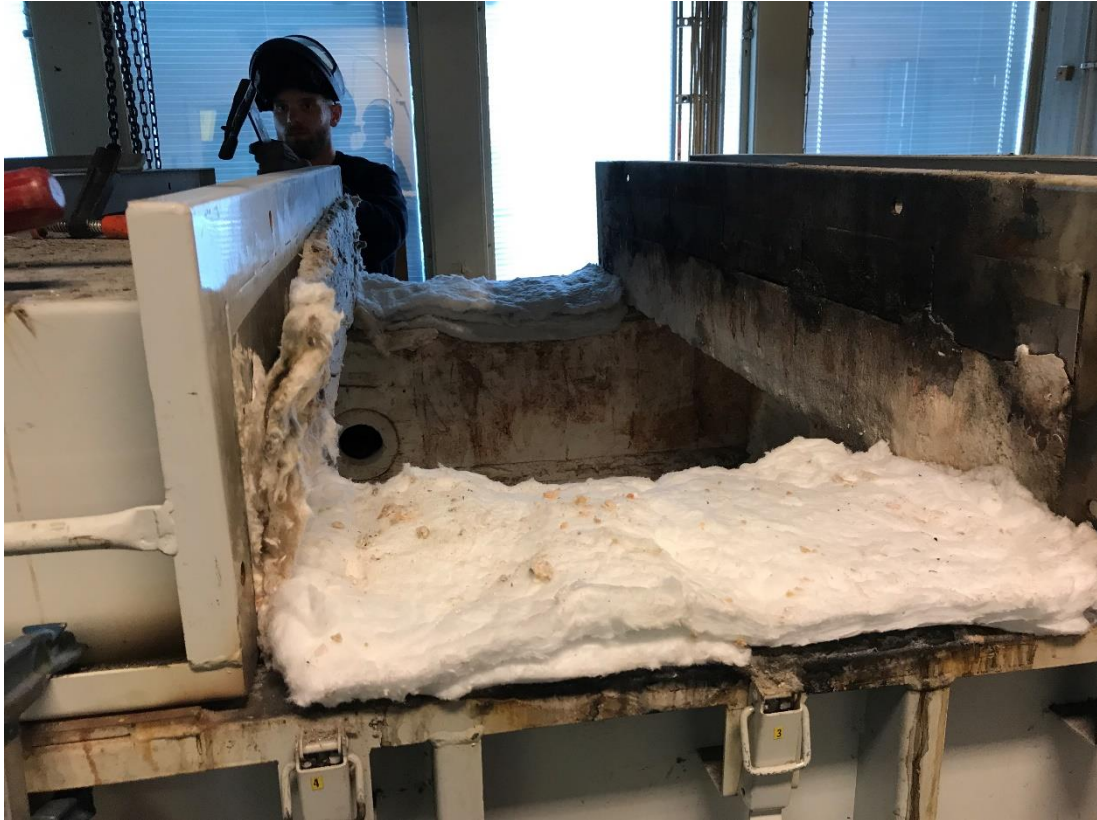
fig. G-17. Typical example for the opening where the test specimens are placed, surrounded by insulation as well as steel beams.
