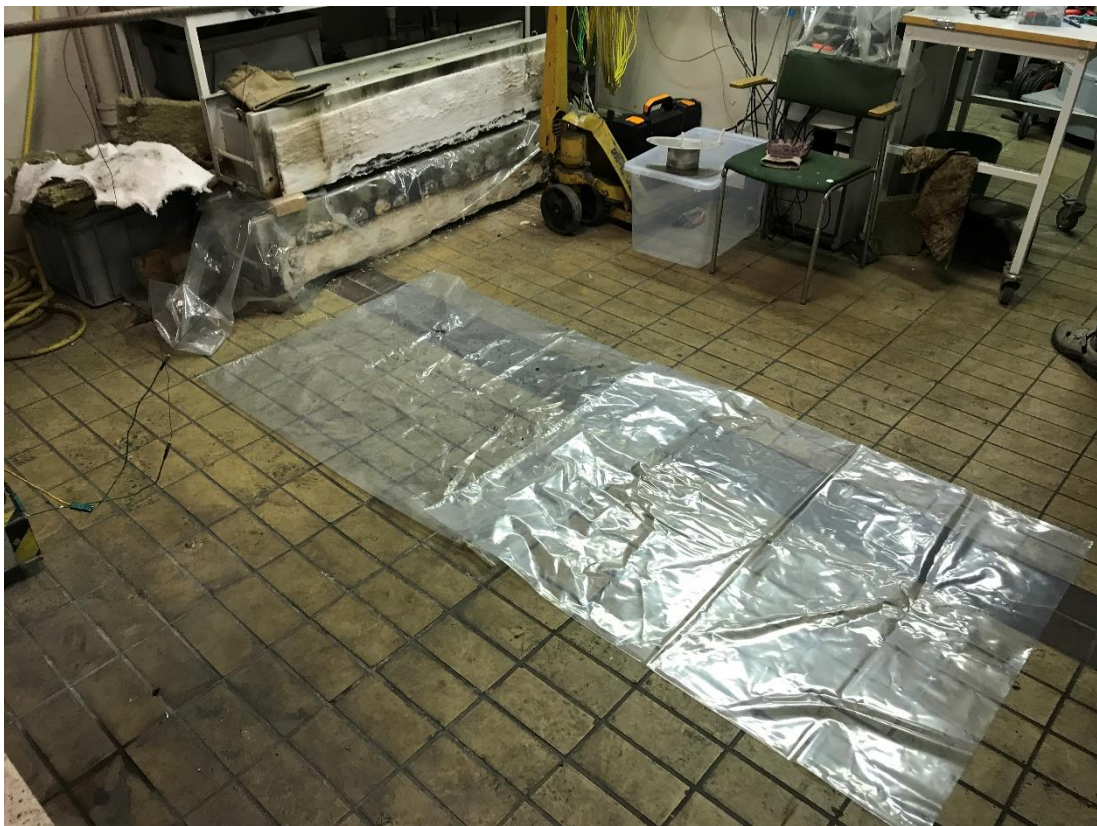
fig. G-24. Plastic bags located in front of the furnace for collection of falling charcoal from specimens during lift off from the furnace.
