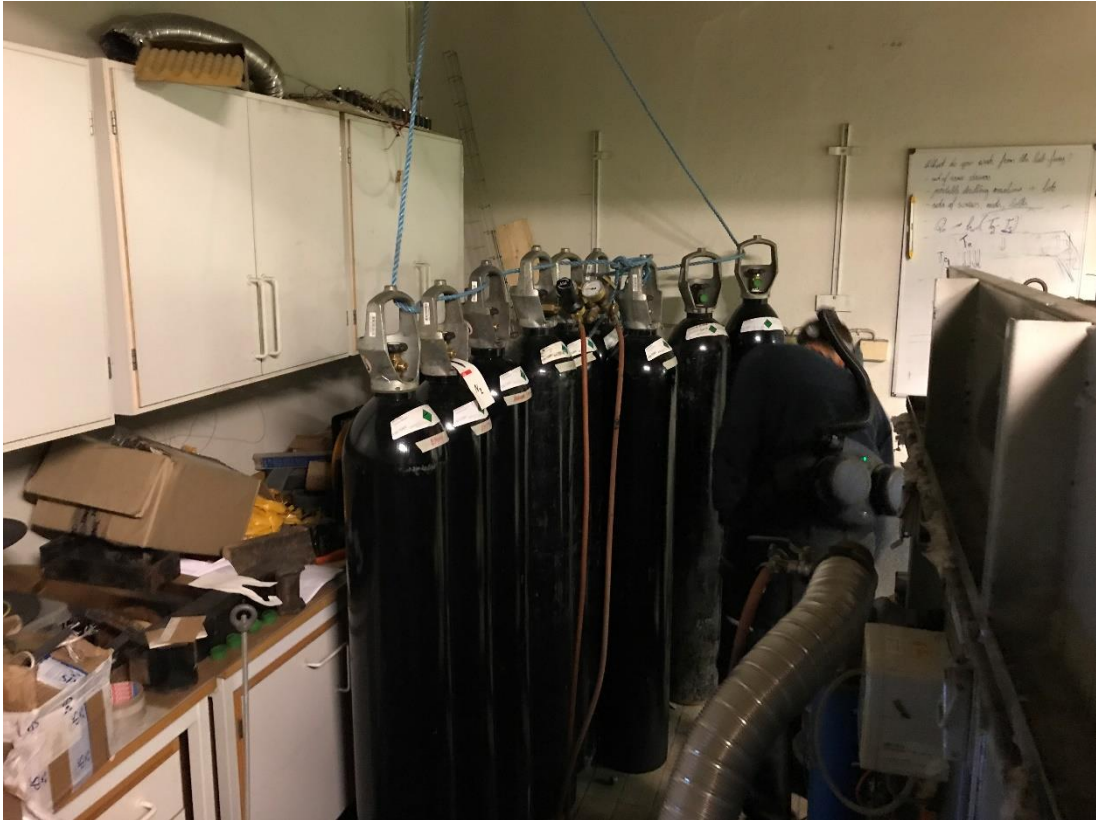
fig. G-21. Nitrogen bottles placed on line for easy access and use during execution of the tests.
