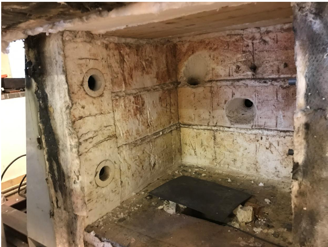
fig. G-16. Inside view of the furnace showing burners, observation tube, exhaust as well as a specimen mounted on top of the furnace.
