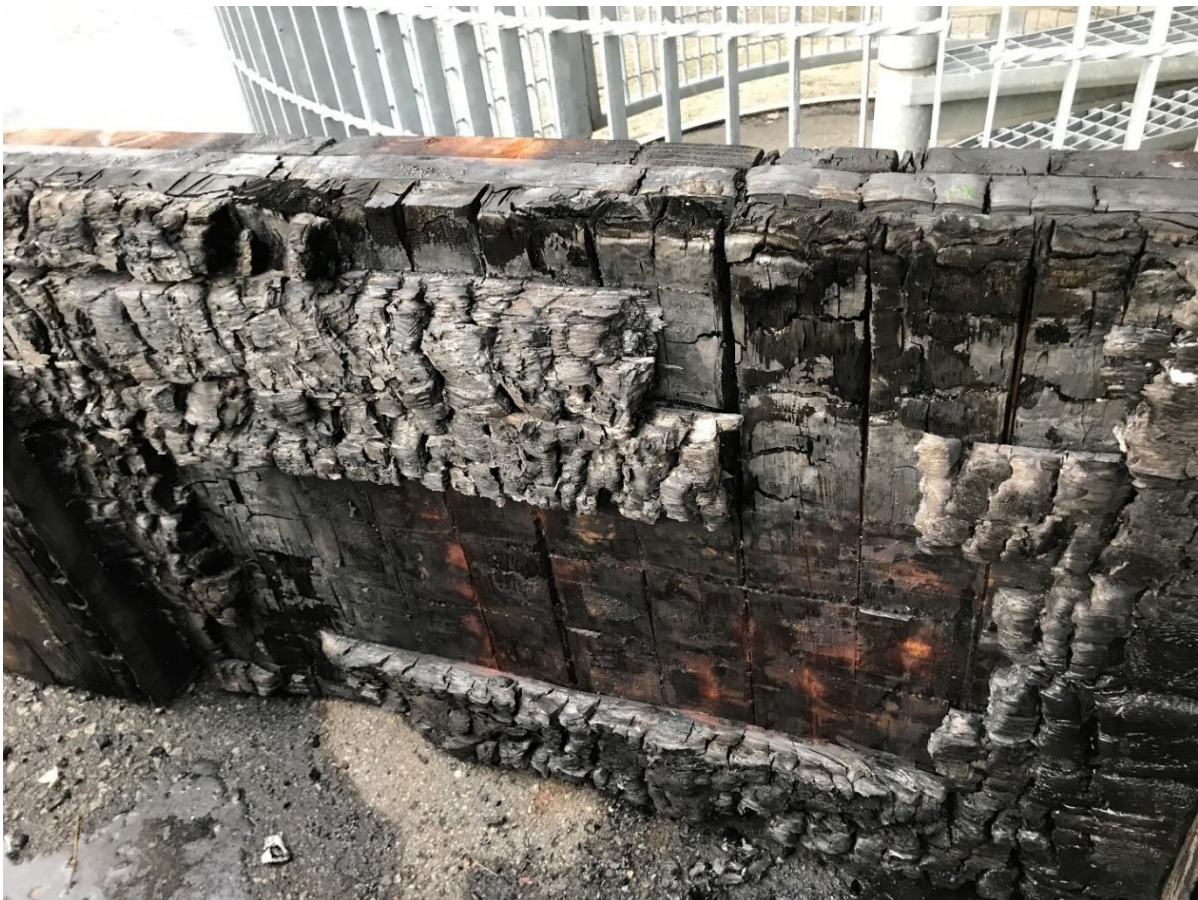
fig. G-10. Specimen PUR-A2 the day after test. The entire first lamella is missing, as it delaminated during the test. Larger portions of the second lamella are missing, exposing fresh wood underneath. Some of these pieces delaminated in the furnace, others fell off after removing the specimen from the furnace.
