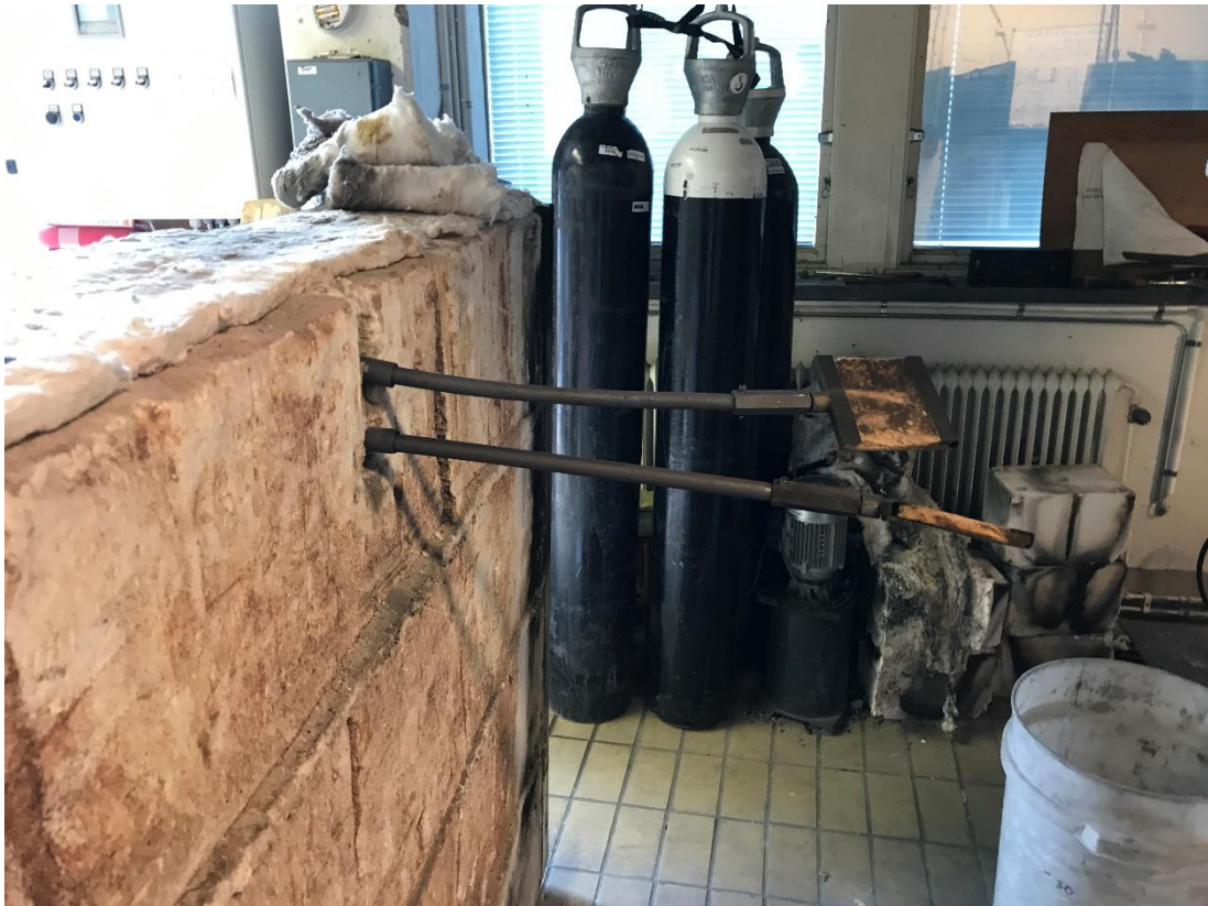
fig. G-19. Plate thermometers placed on the furnace door. Missing from the picture is a thermocouple mounted in the vicinity of the plate thermometer collecting data of the gas temperature.
