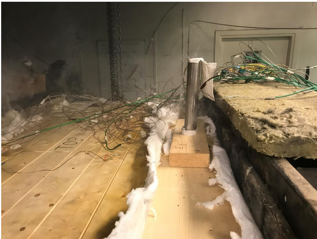
fig. G-28. Location of the heat flux meter while inside the furnace..
