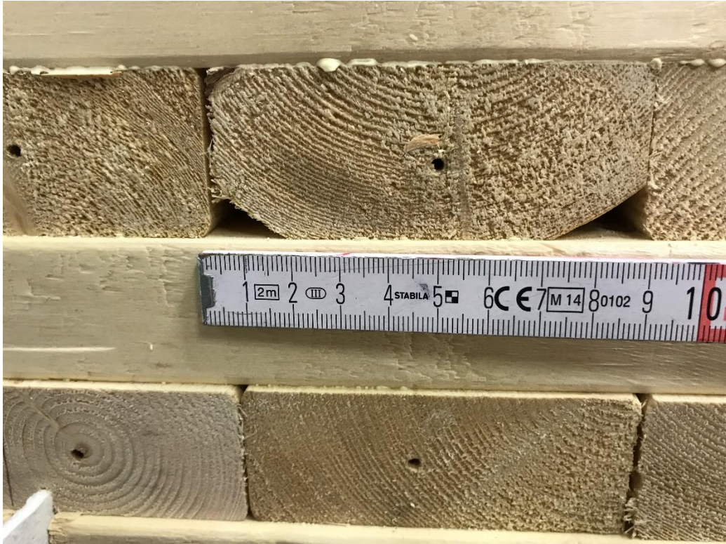
fig. G-7. A board of poor quality in the second lamella from the top of specimen EPI-1, resulting in two openings in the front side.
