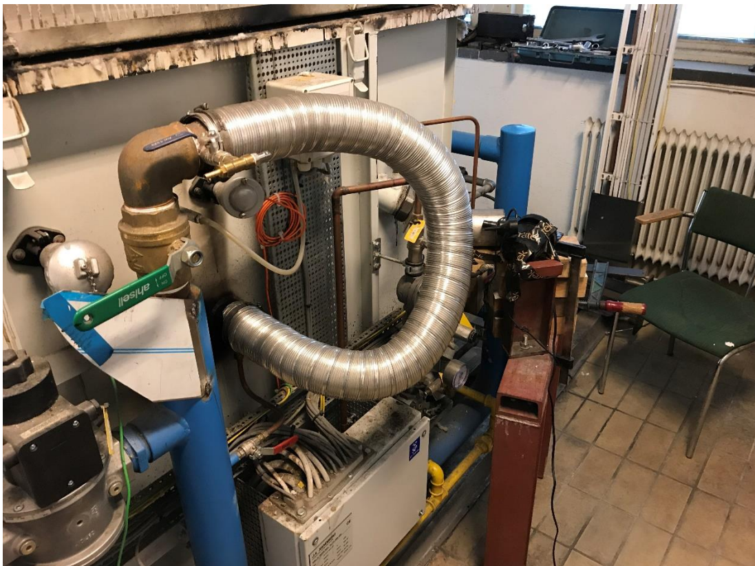
fig. G-20. On the left-hand side of the picture the inflow of air and nitrogen setup can be observed. Next to this setup on the right side the video camera setup can be slightly seen.
