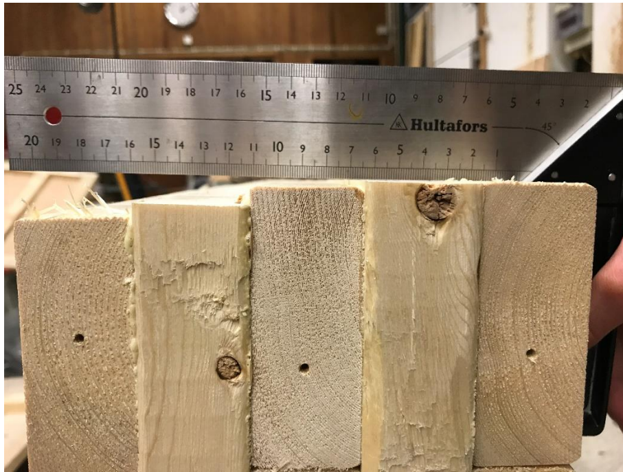
fig. G-9. Section view of specimen PUR-B2. No specimen was entirely plane shaved, and some were in fact extremely uneven like shown in this picture.
