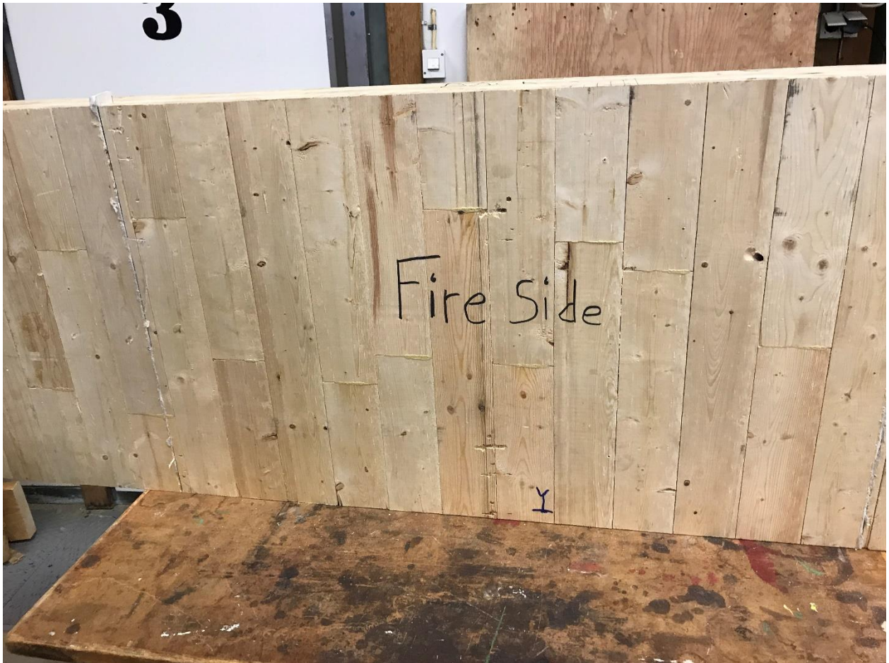
fig. G-1. The fire exposed side of specimen PUR-A1. As these specimen were cut from larger original element from the previous full-scale test, the boards of each lamella were not evenly distributed.
