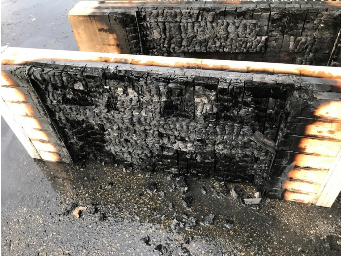
fig. G-12. The EPI-1 specimen the day after testing. Larger pieces of the first lamella fell off during the test, but complete delamination was not observed.
