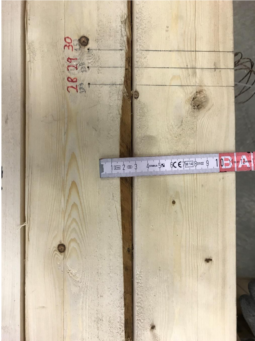
fig. G-2. Top side of EPI-1 specimen. Some boards of the specimen were of very poor quality, with defects such as the one above.
