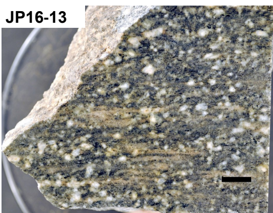
Fig. 16. Plagioclase phenocrystic mesocratic rock from Lammhultsvägen at Skärslund (sample JP16-13). (A) The wet hand sample shows plagioclase phenocrysts, elongate silica-rich domains and a foliated texture. (B) Scan of thin-section cut parallel to the lineation, showing foliae of hornblende, biotite, and opaque minerals. The matrix surrounding the plagioclase phenocrysts consist of quartz, K-feldspar and metamorphic plagioclase. (C) Scan of thin-section cut perpendicular to the lineation.
