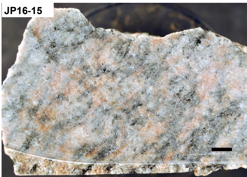
Fig. 18. Meta-granite from Möcklehult (sample JP16-15). Scale-bars are 1 cm. (A) Hand specimen of the rock illustrating the relict medium to coarse grain-size with dark foliae. (B) Scanned thin-section cut parallel to the lineation. Elongate augen of K-feldspar and plagioclase are surrounded by foliae of hornblende, biotite, opaques, and titanite. Zircon, apatite, and epidote occur as accessory phases. (C) Scanned thin-section cut perpendicular to the lineation. The plagioclase and K-feldspar augen are more visible from this angle.
