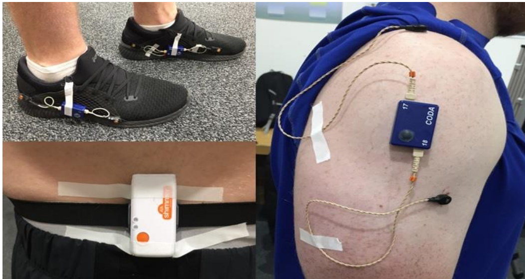
Figure 23 - T.L. Codamotion markers on the feet. B.L. Shimmer unit on the lower back. R. Codamotion markers on the shoulder
