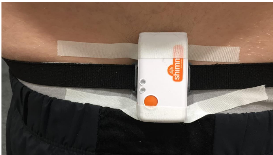
Figure 22 - The Shimmer unit attached to one of the participants
