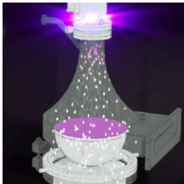
Figure 2.3: Equipment diagram of remote ICP plasma chamber with downstream sample chamber. Bright pink represents creation of plasma. Pink dots represent radicals (N, H). White dots represent inert carrier Ar gas. This remote configuration, with its associated lack of accelerated ion bombardment, is considered imperative for achieving minimal damage to NWs. Reproduced from Cambridge NanoTech Fiji F200 system manual.[90]
