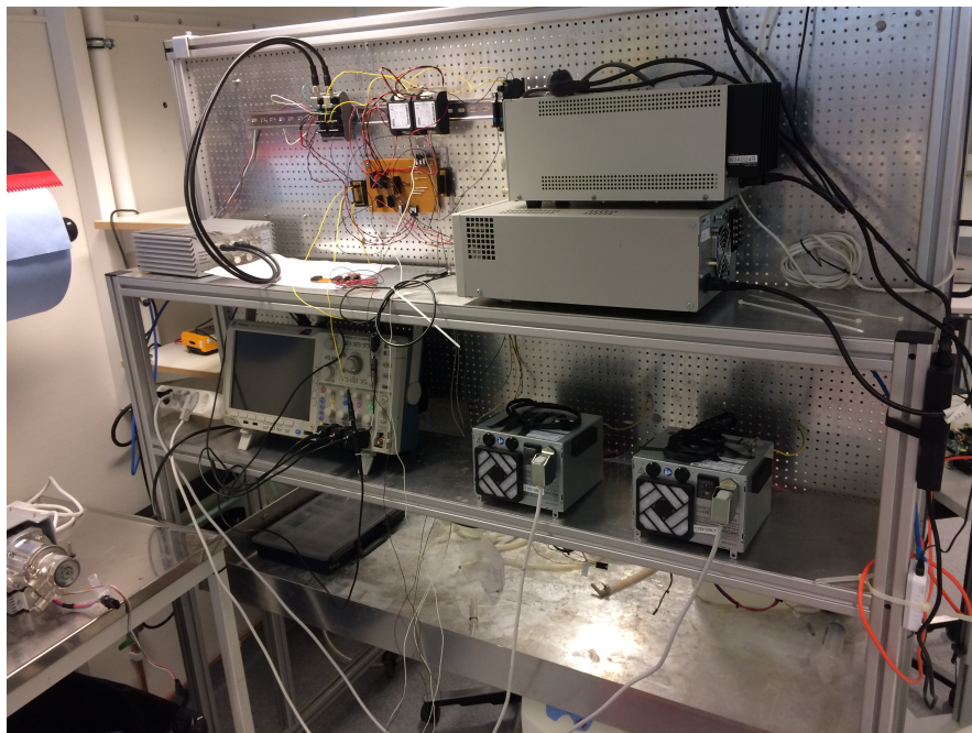
Figure 6.18 Back side of the rig, top shelf: Speedgoat, power supplies and electronics to measure the sensors and control the motors and drain valve. Bottom shelf: power supplies connected to the motors.
