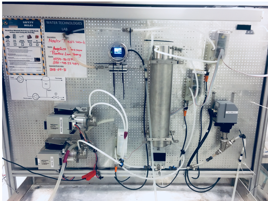
Figure 6.16 The rig built at Baxter Lund AB, with RO-membrane, pumps, pipes, flowmeter, measurement sensors and valves.
