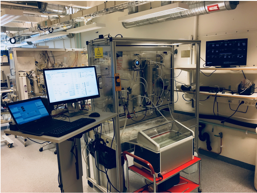
Figure 6.17 The full setup built at Baxter Lund AB, with Simulink implementation, GUI, display and water bath.
