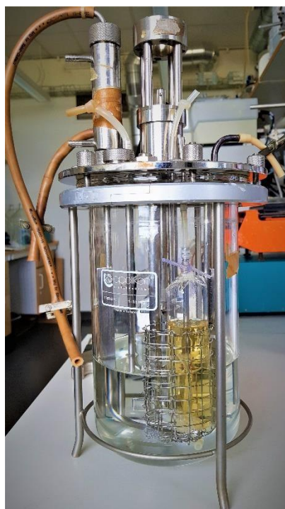
Figure 19: The prototype with a cage and dialysis tubing for co-culturing of L. reuteri and P. copri with media in the dialysis tubing and water inside a 3L single-walled glass fermenter.
