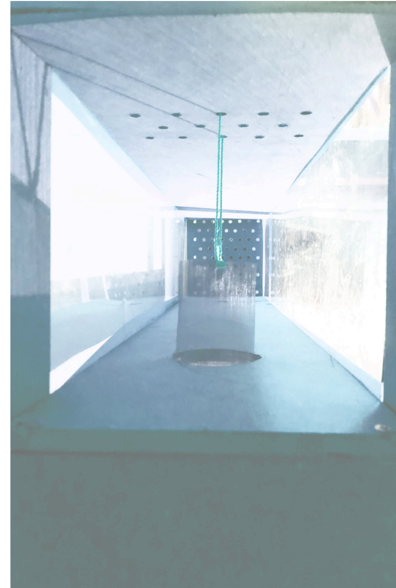
Image 1: Mesh fabric in wind tunnel (Richter 2020)
