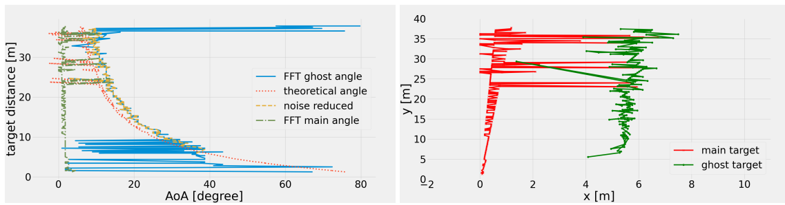
(a) The angle of arrival of the main and ghost target (b) The Cartesian coordinates of both targets. (the latter also with its theoretical angle to discern erroneous classification).
